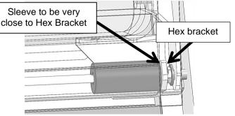
1.16 Once the torsion spring is in position (and the tailgate remaining ajar) slide the Sleeve over the Blades and Hex Stud, the Sleeve should go very close to the Hex Bracket.
