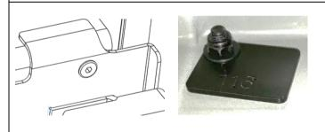
1.19 Tail gate in lowered position: Tighten the 6151882 M8 Ultra Thin Head Screw & M8 Nyloc nut which was left loose on step 1.7. **Torque to 10Nm.**
