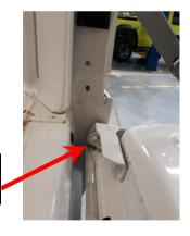
1.3 Remove the hinge bolt from the RHS of the tailgate and discard.
