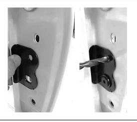
2.8 Remove the Bracket and reassemble using the 3195150 Plate on the inside of the Tail Light cavity to sandwich the panel.
