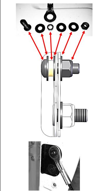
2.3 Fasten the eye end of the 6821348 Cable through this hole as shown using an 6151464 M8 Button Head Screw, 3x M8 Washers, 5848468 Spacer and Nyloc Nut.
