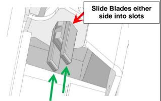
1.12 Slide in the 3193801 support blades through the hex bracket above the large flat surfaces of the Hex Bolt. (Blades should hold in position)
