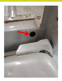
1.1 Open the tailgate. Remove and discard the rubber bung (if fitted) on the body of the tub near the RH Hinge.
