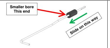
1.13 At the free end of the Torsion Spring, place the sleeve over the Spring. (Insert the sleeve through the smaller bore into the Torsion Spring.)
