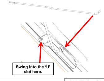
1.11 Taking the bent end of the Torsion Spring, feed it into the Threaded Bush and swing it into the 'U' slot of the Bracket.
