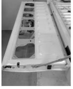
1.8 Remove the Tailgate Inspection Panel to enable access to the inside of the tailgate. (Retain all parts to refit at a later stage.)
