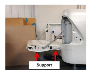
1.2 Support the tailgate in the open position to avoid any chance of the tailgate falling as hinge bolts are to be removed as part of installing the Tailgate Lift Assembly.
